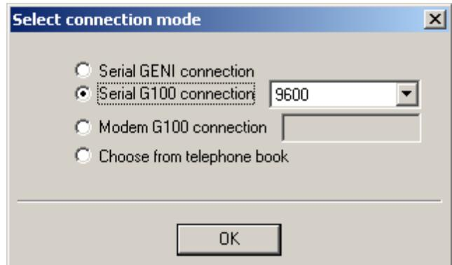
If two or more COM ports are available, a selection box appears. Select the COM port to which the PC Tool link is connected.
