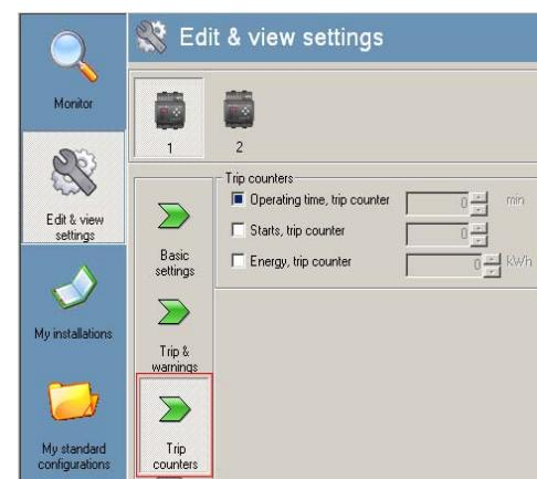
To preset a counter, write-enable the field by putting a check mark in the check box and enter a value.
