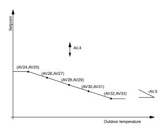
Five-point temperature curve. Y axis: Setpoint [°C]. X axis: Outdoor temperature [°C].
