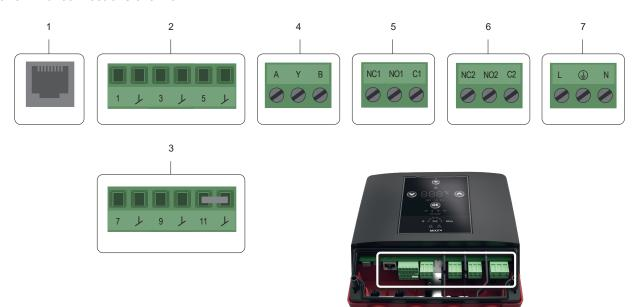
Pos. Description 1 Ethernet RJ45 (BACnet IP, Modbus TCP) Configurable I/O 2 3 Configurable I/O 4 RS485 transceiver (BACnet MS/TP, Modbus RTU) Relay 1 5 6 Relay 2 Mains supply. Carry out the electrical connection and protection according to local regulations. 7
