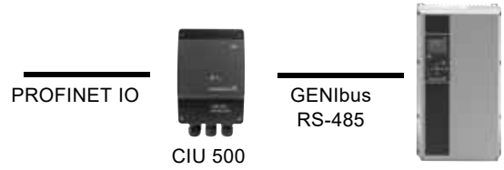
Fig. 4 Example of a CIU 500 solution. The figure shows a CUE-drive for pumps
