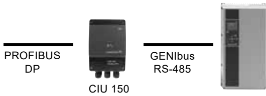
Fig. 2 Example of a CIU 150 solution. The figure shows a CUE-drive for pumps
